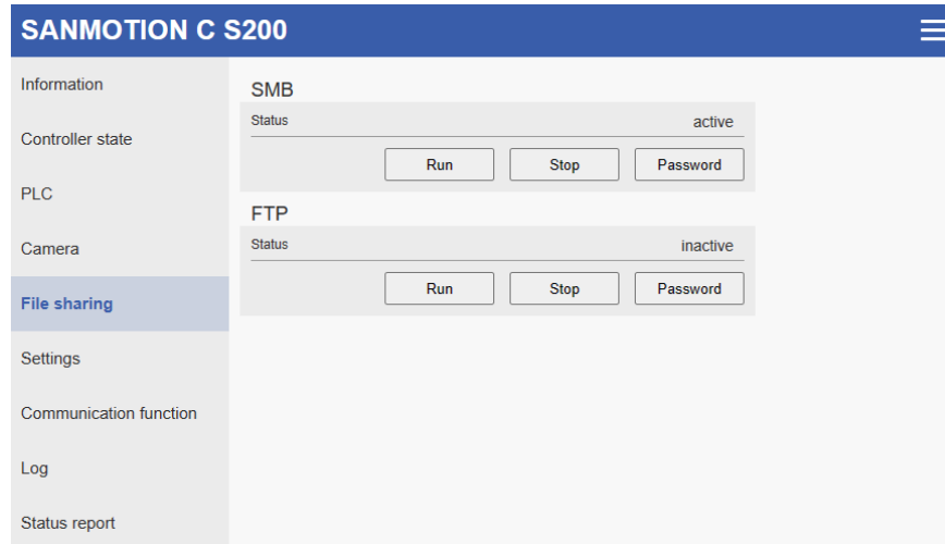
Fig.6.48 Enable server from web application
