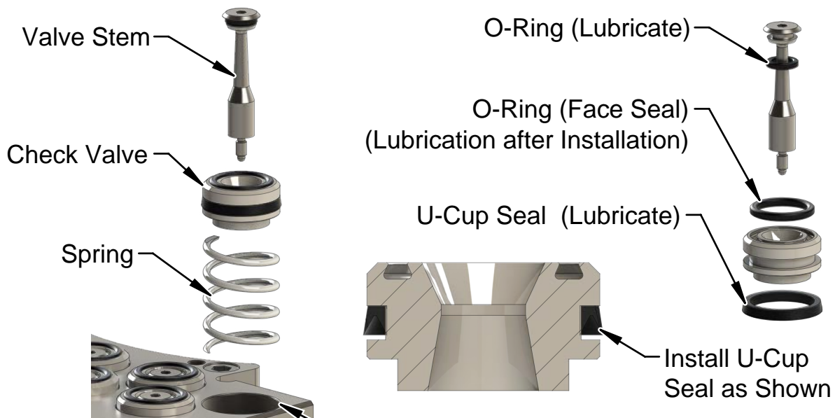
Figure 5.2—Master Self-Sealing Valve Installation
