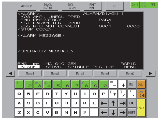
Alarm Diagnosis Monitor
