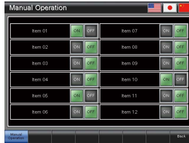
Manual operation (6 patterns) Executes ON/OFF operations of signals (bit devices)
