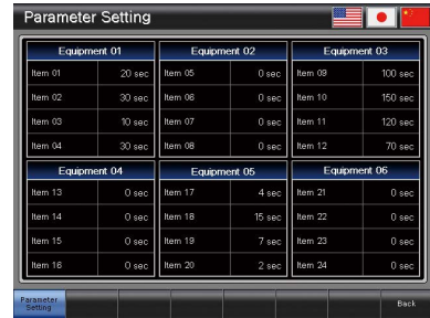
Parameter setting (3 patterns) Displays set items and enables input of set values for various parameters
