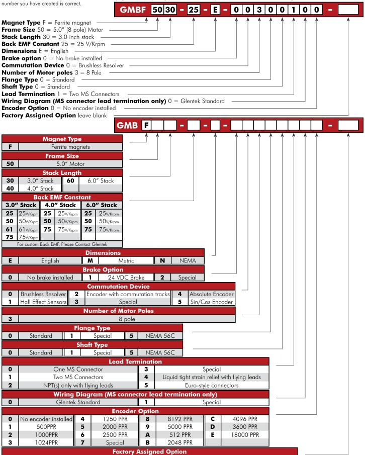
A numerical code will be assigned by Glentek to motors whose specifications vary from the standard configuration
