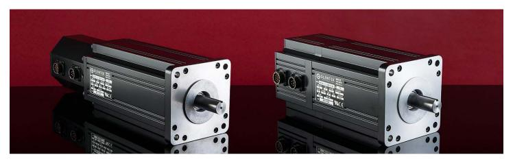
Glentek's GMBF5000 series of high performance, permanent magnet Brushless servo motors utilize traditional ferrite magnets which are ideal for cost sensitive applications. This helps to reduce the mechanical shaft resonance which allows higher servo gains with increased stability. In addition, all frame sizes incorporate skewed stators which provide ultra smooth operation (i.e. low cogging torque) at all speeds.
