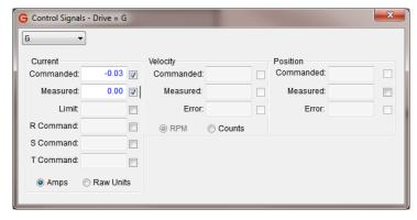
Enter a 0 amp command for *Current (Amps)* on the *Control Panel* window and enable your drive. Verify that the *Commanded* and *Measured* values match (within a margin of error that suits your application). If they do not match, adjust the *Signal Offset* under *Analog Input Setup* in the *Drive Mode* window by the difference of the *Commanded* and *Measured Current* values divided by the *Signal Gain*.
