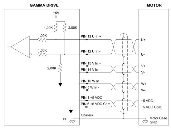
Figure 3-23 Digital Hall Circuit (Differential)
