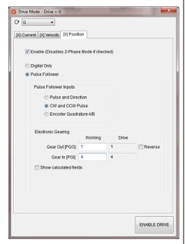
The drive is now set up to accept CW and CCW pulse follower command inputs.
