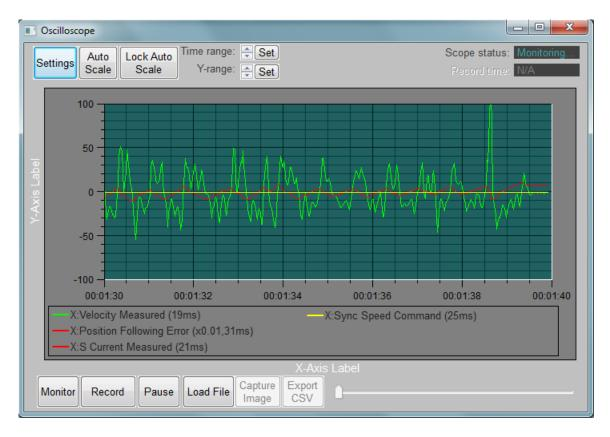
The MotionMaestro Oscilloscope window is a full-featured, real-time data plotter and recorder that provides the following capabilities:
