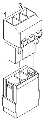
Figure 3-29 Non-UL Stand Alone Motor Output Connector
