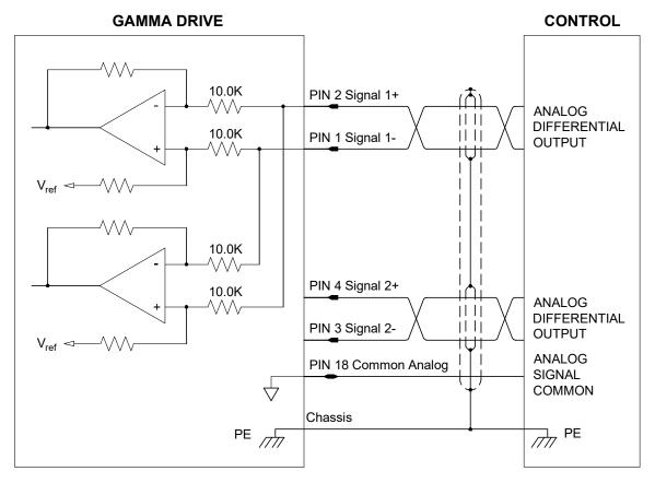
Figure 3-10 Differential Analog Input
