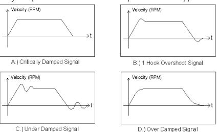
Figure 4-1 Oscilloscope Waveforms
