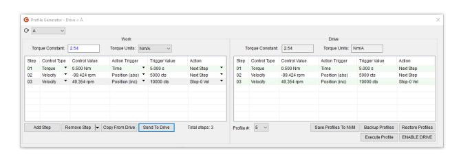
The second and third step will turn the motor until the encoder moves through 5000 counts (from the current encoder count) in the negative direction at -100 RPM and then move in the positive direction through 10,000 encoder counts at 50 RPM.
