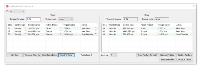
When you first bring up this screen it will give you a single step on the left. As long as the drive is not currently executing a profile, the currently active profile for the drive on the right. If your drive is currently executing a profile, you will be prompted to disable the drive so the profile can be loaded. Your drive may be preloaded with profiles set by the factory based on your use case.
