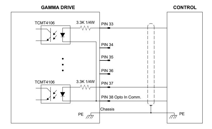
Figure 3-2 Optically Isolated Programmable Digital Input
