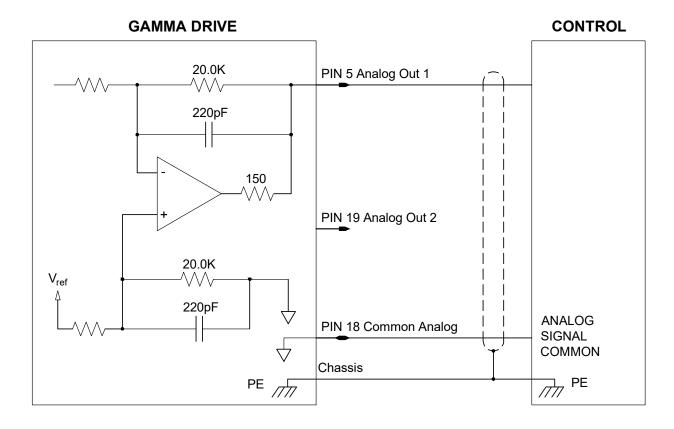
Figure 3-12 Analog Outputs
