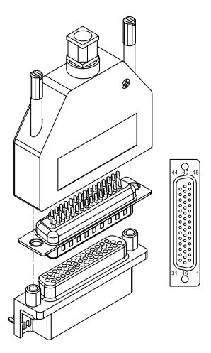
Figure 3-1 44-Pin I/O connector
