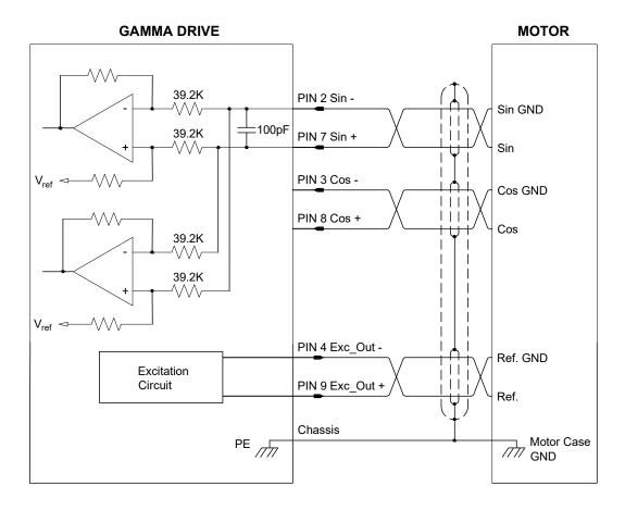
Figure 3-26 Resolver Circuit
