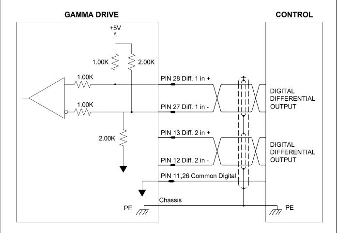
**Figure 3-4 Differential Digital Input**
