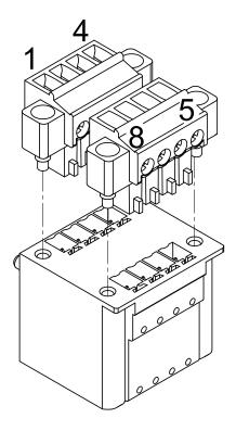
Figure 3-15 Logic Power/Brake/STO Connector (Optional)
