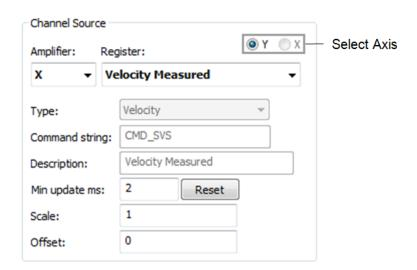
This section displays the settings for the currently selected channel, allowing the user to make changes.
