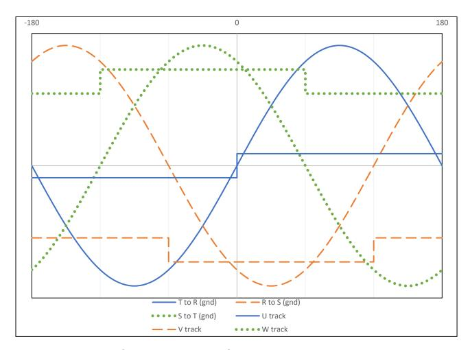
Figure 6-1 Commutation Track Signals and Phase-to-Phase BEMF
