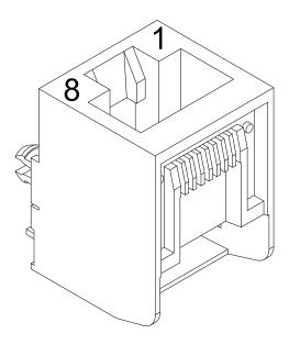
Figure 3-18 RJ45 Mating Connector
