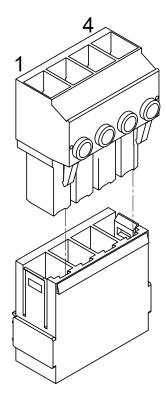
Figure 3-33 Non-UL Stand Alone AC Power Input Connector
