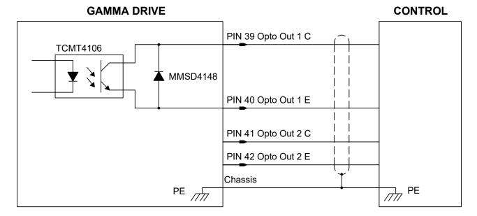
Figure 3-8 Optically Isolated Programmable Digital Output
