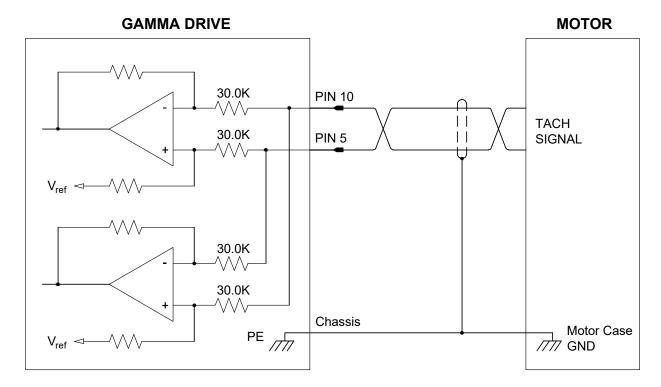
**Figure 3-25 Tachometer Circuit**
