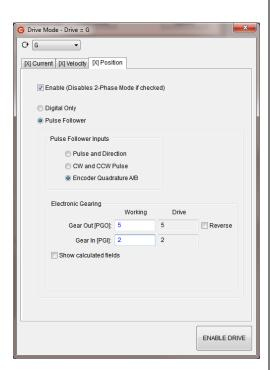
The drive is now set up to accept encoder quadrature A/B command inputs.
