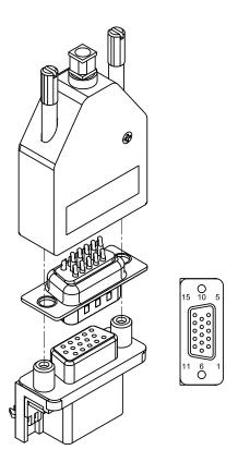
Figure 3-22 Motor Feedback Connector
