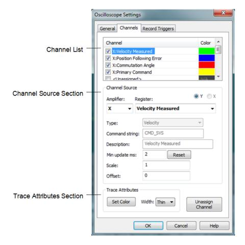
This window sets up the channels that are to be displayed in the oscilloscope plot area and optionally recorded.
