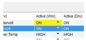
Like most settings in MotionMaestro: The drive does not change until you click the <u>Send to Drive</u> button. After you have tested your settings and are ready to make the changes permanent use the <u>Setup -> Save to NVM</u> menu option to save the settings to permanent memory on the drive.
