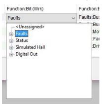
Each category can be expanded by clicking the + sign. In the *Faults* category, the faults you see are a list of the faults that relate to the *Drive Status* window (**Status -> Drive Status...**) and in Table 5-3.
