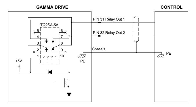
Figure 3-9 Relay Output
