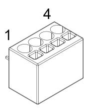
Figure 3-32 UL Stand Alone AC Power Input Connector
