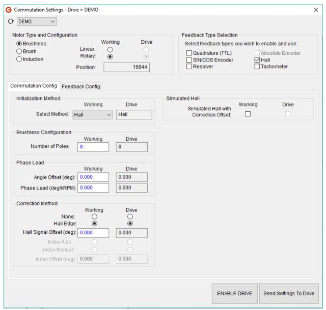
This window is designed to only display relevant information based on the motor type and feedback. As you make changes to the *Motor Type* and *Feedback Type Selection*, the bottom section of the window with the tabbed interface will change and adapt to the selections. This way, options which cannot be used are not shown.
