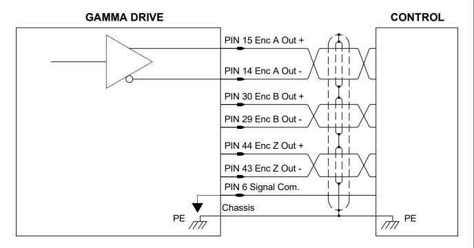
Figure 3-13 Encoder Outputs
