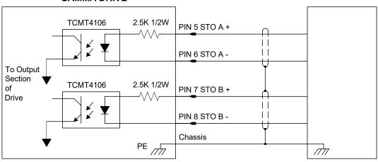
Figure 3-17 STO Input Circuit
