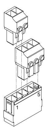
Figure 3-36 Non-UL Module DC Power Input and Motor Output Connector
