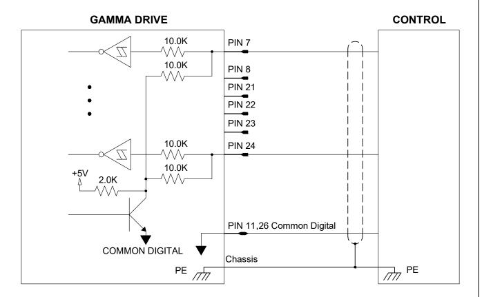
Figure 3-3 Schmitt Trigger Digital Input
