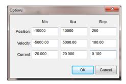
Type 0 into the *Current (Amps)* field and press enter to ensure that the motor will not move when enabled. Enable the drive, then press the >> button to positively increment the current command. Press the button until you see the motor move. Both the *Current (Amps)* and *Actual Velocity (RPM)* values should be positive. If the *Actual Velocity (RPM)* is negative, check the *Tach. Reverse* box.
