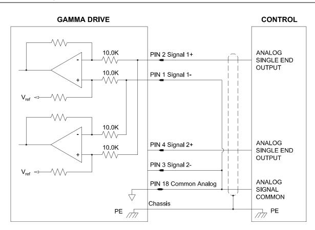
Figure 3-11 Single Ended Analog Input
