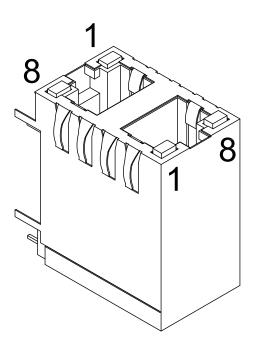
Figure 3-20 RJ45 Double Mating Connector
