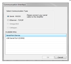
5. A notification will let the user know which type of drive is connected. After verifying the correct drive(s) is/are shown click <u>OK</u>.
