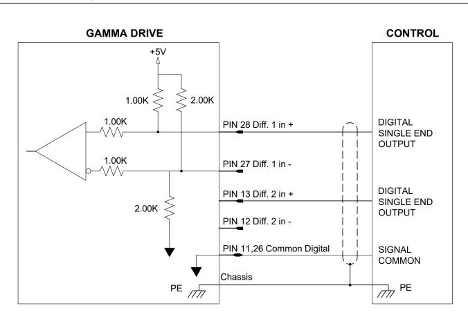
Figure 3-5 Differential Digital Input Single Ended
