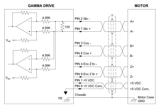
Figure 3-27 Sin/Cos Encoder Circuit
