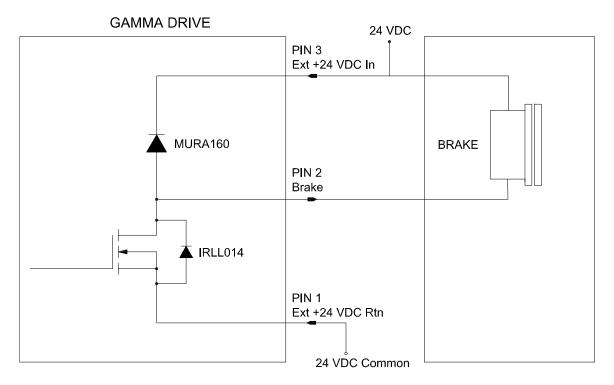
Figure 3-16 Brake/Stop Sequence Internal Circuit
