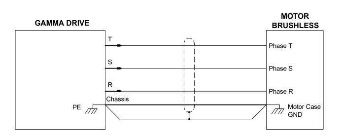
Figure 3-30 UL and Non-UL Stand Alone Motor Output Brushless
