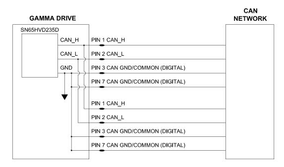
**Figure 3-21 CANopen Connection Diagram**
