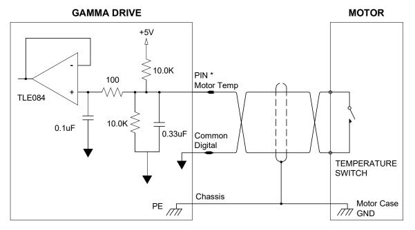
Controller I/O: PIN 20 pair with PIN 11 or 26 - Common Digital Motor Feed Back: PIN 11 - pair with Pin 6 - Common
