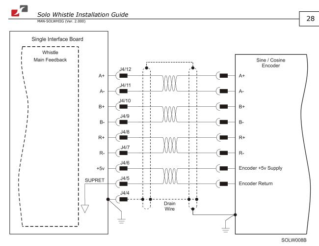
Figure 6: Main Feedback – Interpolated Analog (Sine/Cosine) Encoder Connection Diagram
