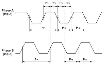
Figure 49: Auxiliary Feedback - Encoder Phase Diagram
