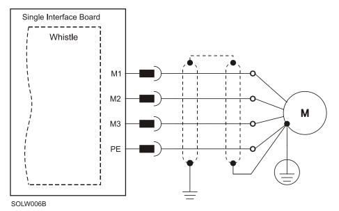
Figure 26: AC Motor Power Connection Diagram
