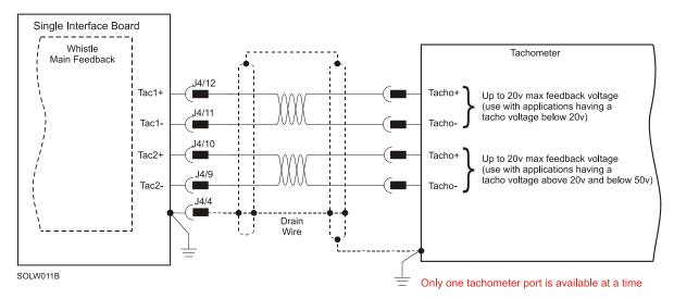
Figure 11: Main Feedback – Tachometer Feedback Connection Diagram for Brush Motors
