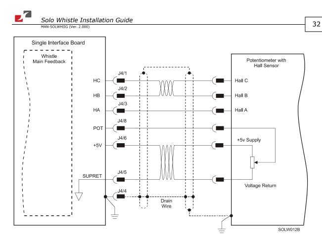
Figure 12: Main Feedback – Potentiometer Feedback with Digital Hall Sensor Connection Diagram for Brushless Motors
