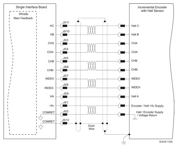
Figure 29: Main Feedback- Incremental Encoder with Digital Hall Sensor Connection Diagram
