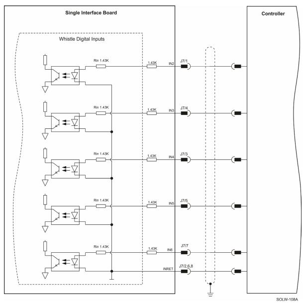
Figure 40: Digital Input 24 Connection Diagram
