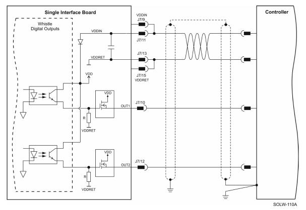
Figure 42: Digital Output 24 V Connection Diagram
