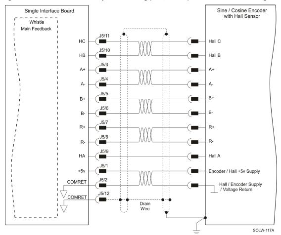
Figure 31: Main Feedback – Interpolated Analog (Sine/Cosine) Encoder with Digital Hall Sensor Connection Diagram
