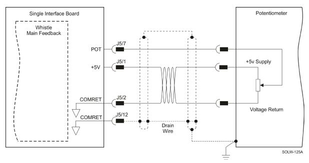
Figure 37: Main Feedback – Potentiometer Feedback Connection Diagram for Brush Motors and Voice Coils
