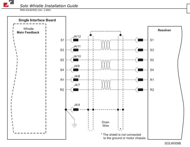
Figure 8: Main Feedback – Resolver Connection Diagram
