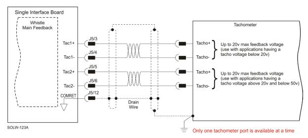
Figure 35: Main Feedback – Tachometer Feedback Connection Diagram for Brush Motors
