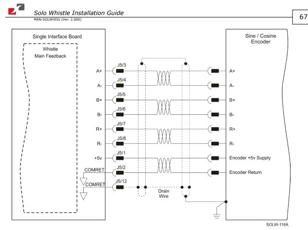
Figure 30: Main Feedback – Interpolated Analog (Sine/Cosine) Encoder Connection Diagram
