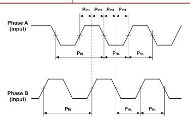
Figure 48: Auxiliary Feedback - Encoder Phase Diagram
