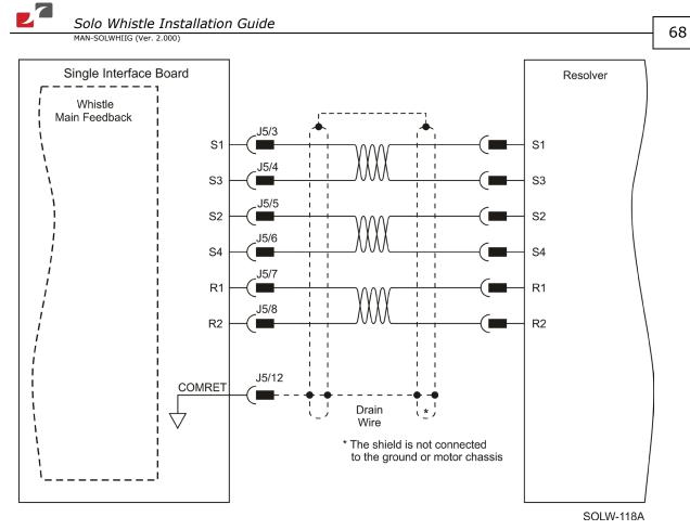
Figure 32: Main Feedback – Resolver Connection Diagram
