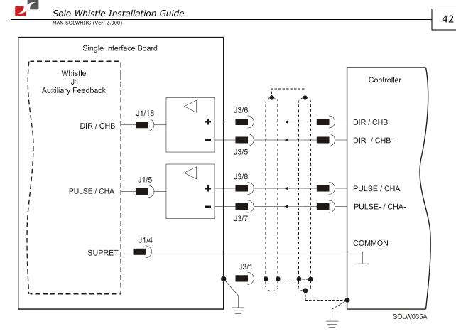
Figure 17: Pulse-and-Direction Diagram
