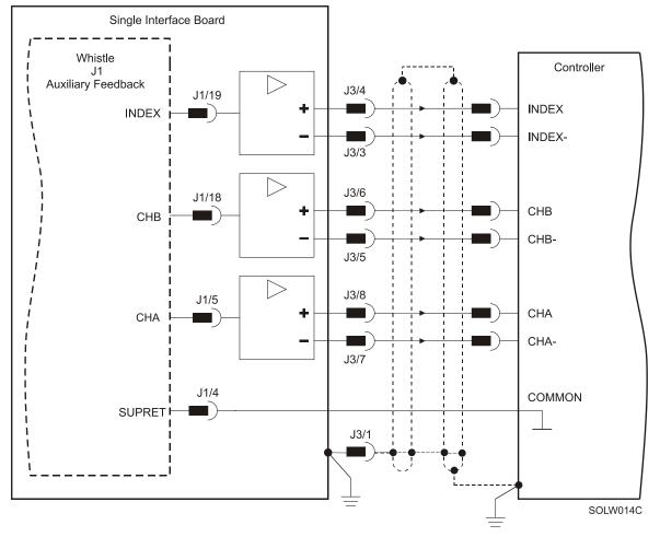
Figure 14: Emulated Encoder Differential Output Diagram
