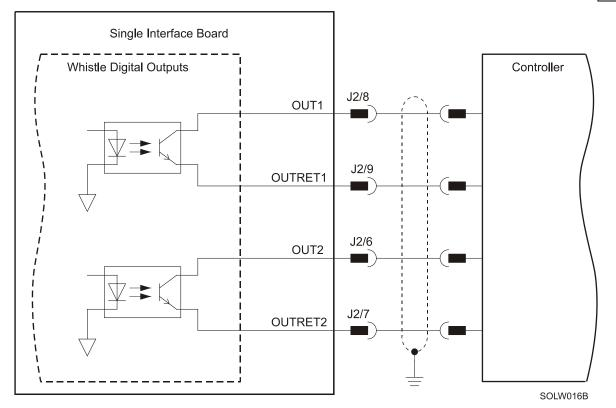
Figure 21: Digital Output Connection Diagram
