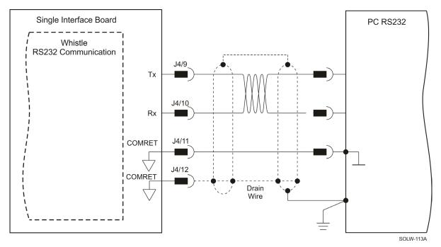
Figure 45: RS-232 Connection Diagram
