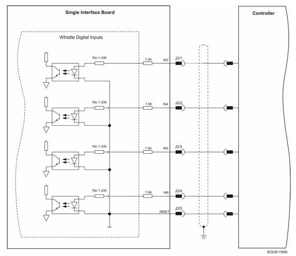
Figure 19: Digital Input 24 Connection Diagram
