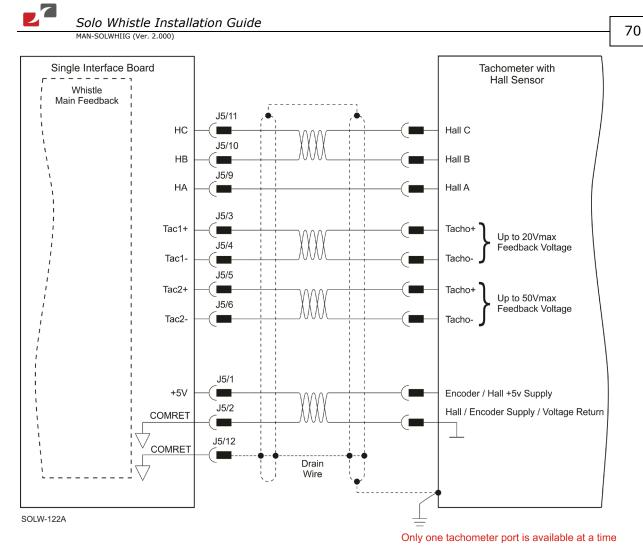
Figure 34: Main Feedback – Tachometer Feedback with Digital Hall Sensor Connection Diagram for Brushless Motors
