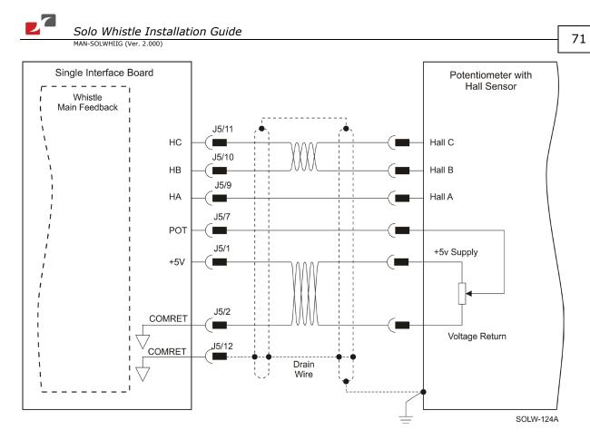
Figure 36: Main Feedback – Potentiometer Feedback with Digital Hall Sensor Connection Diagram for Brushless Motors
