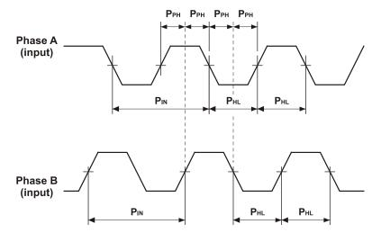
Figure 47: Main Feedback - Encoder Phase Diagram
