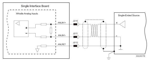
Figure 23: Analog Input with Single-Ended Source
