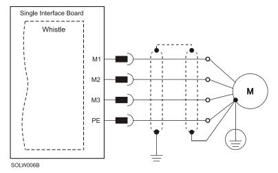
Figure 3: AC Motor Power Connection Diagram
