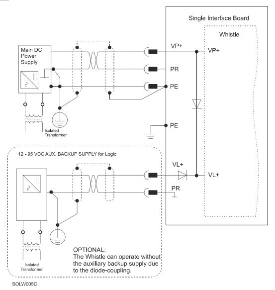
Figure 27: Main & Auxiliary Power Supply Connection Diagram
