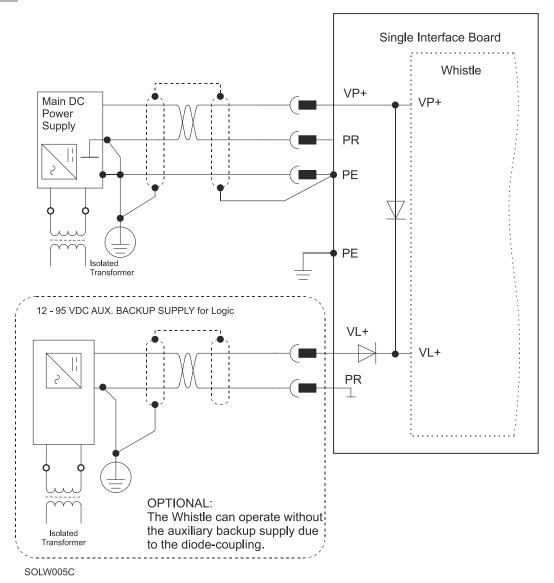
Figure 4: Main & Auxiliary Power Supply Connection Diagram
