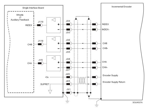
Figure 16: Differential Auxiliary Encoder Input Option Diagram
