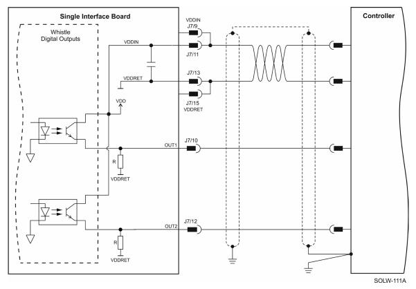
Figure 43: Digital Output 5 V Connection Diagram
