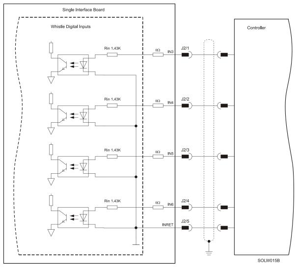
Figure 18: Digital Input 5 V Connection Diagram
