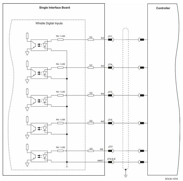
Figure 39: Digital Input 5 V Connection Diagram
