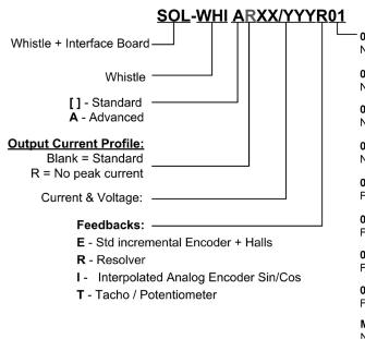
**01 -** 24 VDC (Digital Inputs), Motor Phase **Connector**, Network Position + Velocity (CANOpen)
