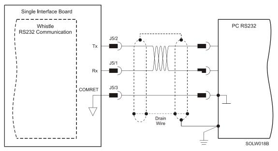
Figure 24: RS-232 Connection Diagram
