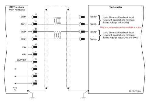
Figure 17: Main Feedback – Tachometer Feedback Connection Diagram for Brush Motors
