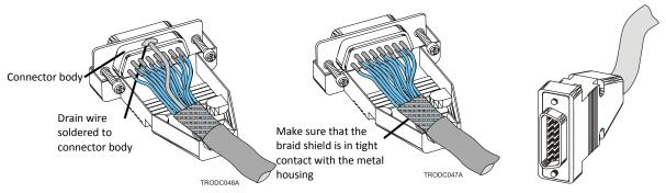
Figure 12: Feedback and Control Cable Assemblies
