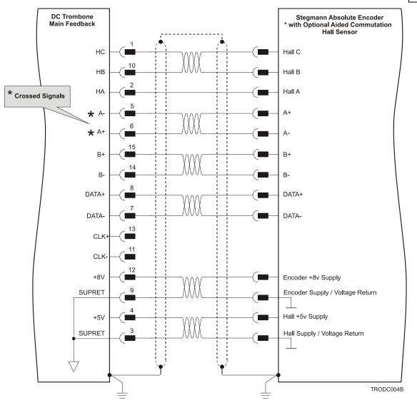
Figure 20: Main Feedback – Stegmann Feedback Connection Diagram
