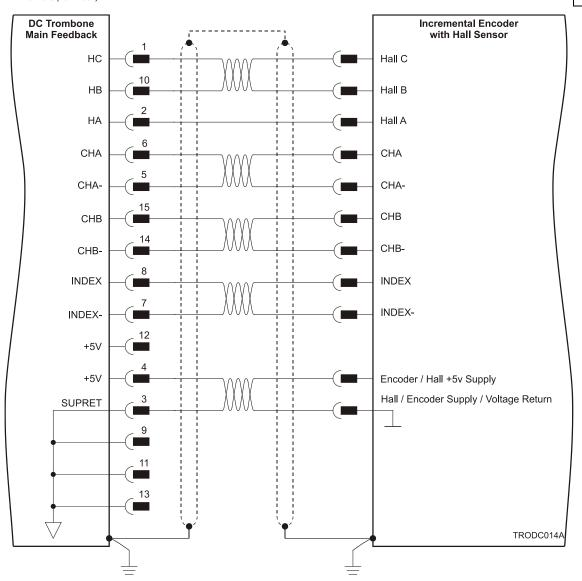
Figure 13: Main Feedback- Incremental Encoder Connection Diagram
