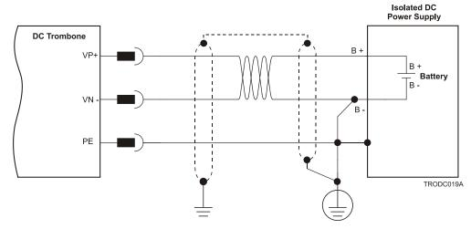
Figure 10: Battery Connection Topology
