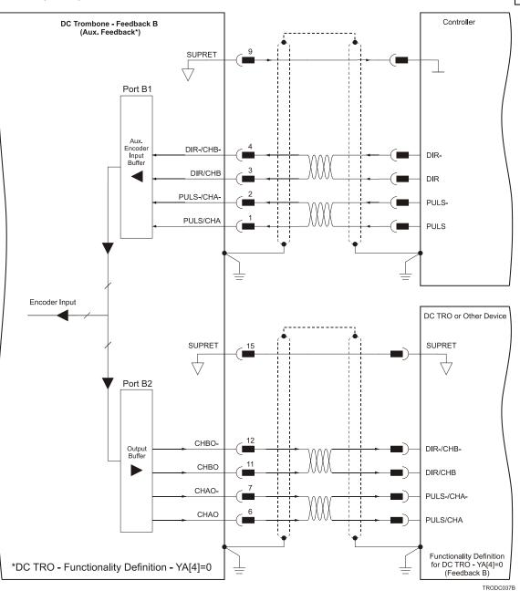
Figure 24: Differential Pulse-and-Direction Input Option on FEEDBACK B - Connection Diagram
