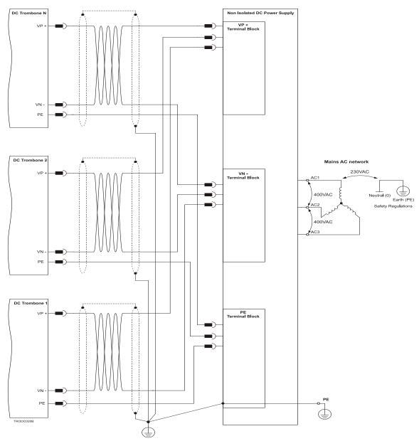
Figure 9: Non-Isolated Three-Phase multiple Connection Topology
