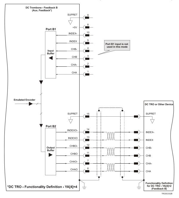
Figure 22: Emulated Encoder Output on FEEDBACK B - Connection Diagram
