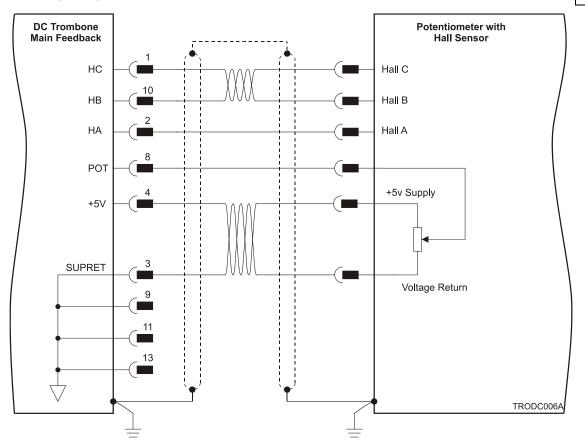
Figure 18: Main Feedback – Potentiometer Feedback with Digital Hall Sensor Connection Diagram for Brushless Motors
