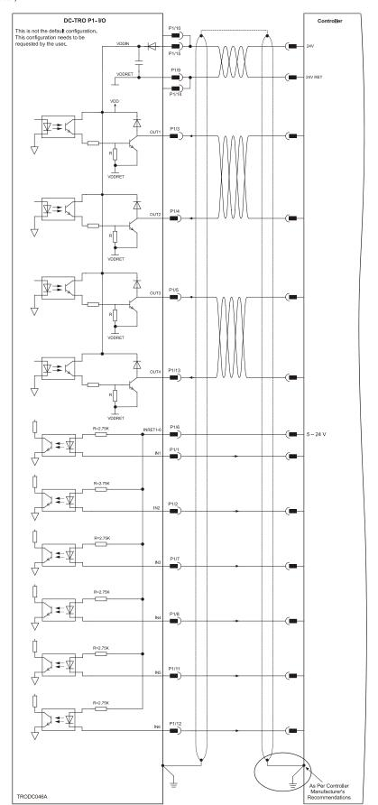
Figure 26: Digital Output (as Sink Configuration) & Input (as Source Configuration) P1 -Connection Diagram
