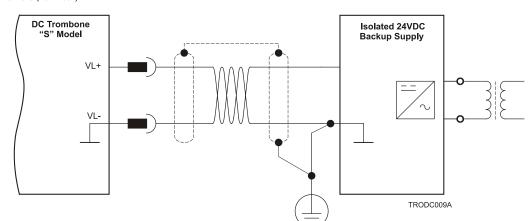
Figure 11: Auxiliary 24 VDC Backup Supply Connection Diagram
