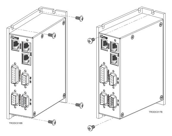
Figure 2: Mounting the DC Trombone with L-shaped Heat-sink
