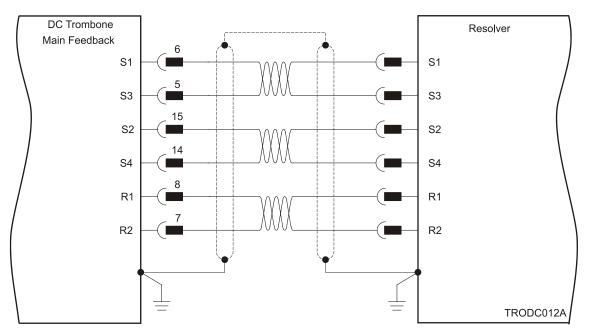
Figure 15: Main Feedback – Resolver Connection Diagram
