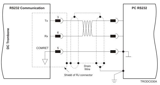
Figure 28: RS-232 Connection Diagram
