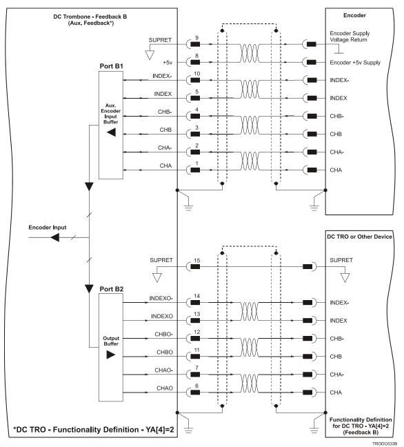
Figure 23: Differential Auxiliary Encoder Input Option on FEEDBACK B - Connection Diagram
