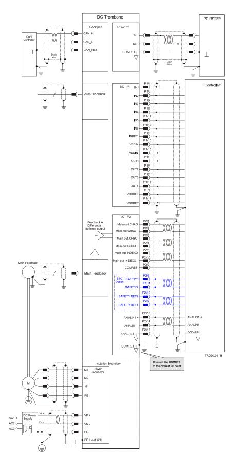
Figure 5: DC-DC Trombone Connection Diagram – 400 V without Backup Functionality
