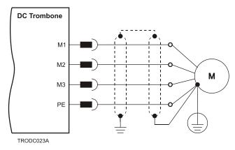
Figure 6: AC Motor Power Connection Diagram
