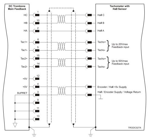
Figure 16: Main Feedback – Tachometer Feedback with Digital Hall Sensor Connection Diagram for Brushless Motors
