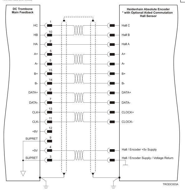
Figure 21: Main Feedback – Heidenhain Feedback Connection Diagram
