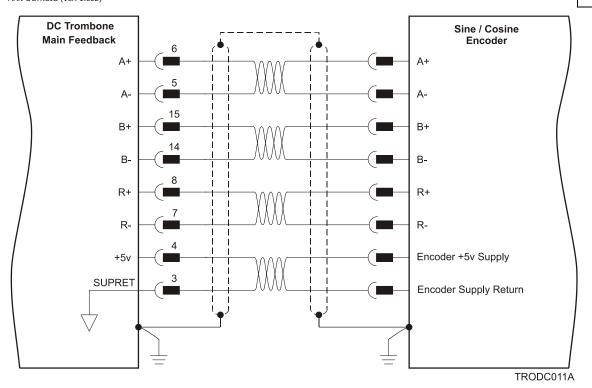
Figure 14: Main Feedback – Interpolated Analog Encoder Connection Diagram
