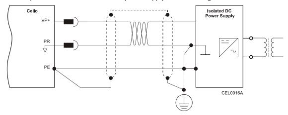
**Figure 6: Main Power Supply Connection Diagram**
