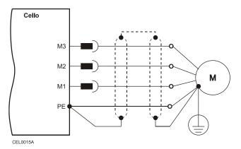
Figure 5: AC Motor Power Connection Diagram
