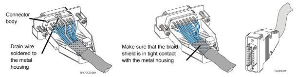
**Figure 8: Feedback and Control Cable Assemblies**
