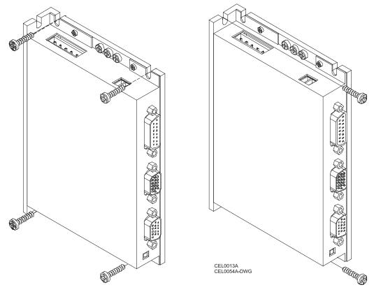
Figure 3: Mounting the Cello
