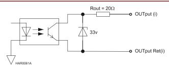
Figure 29: Digital Output Schematic
