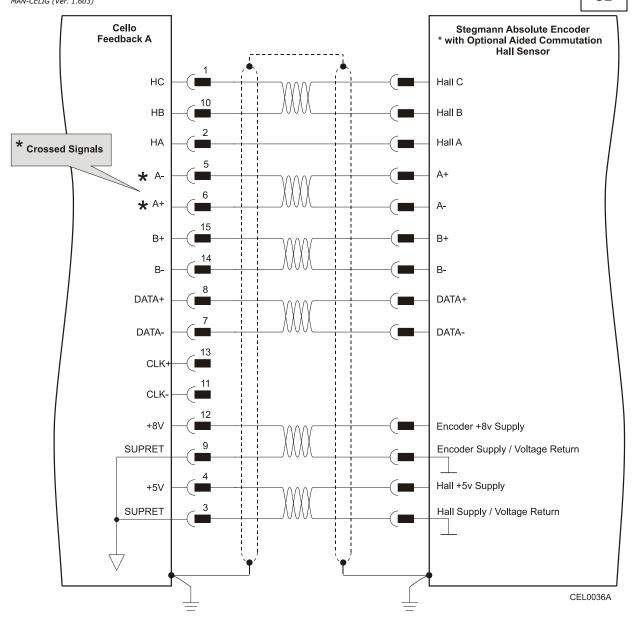
Figure 16: Main Feedback – Stegmann Feedback Connection Diagram
