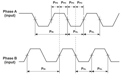
Figure 27: Encoder Phase Diagram
