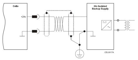
Figure 7: Backup Supply (24v) Connection Diagram
