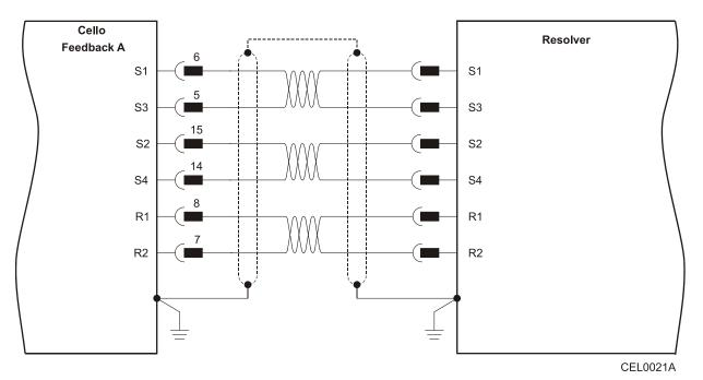
Figure 11: Main Feedback - Resolver Connection Diagram
