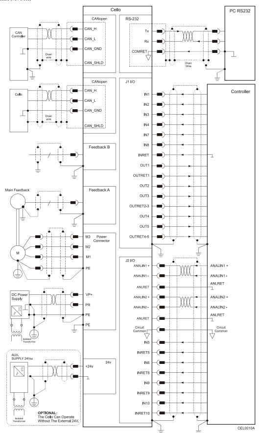
**Figure 4: Cello Detailed Connection Diagram**
