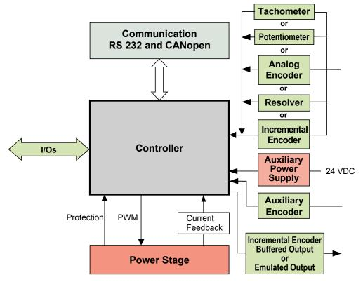
Figure 1: Cello System Block Diagram
