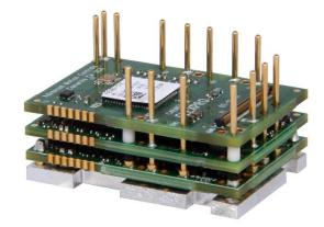
The **FE060-10-EM** is a FlexPro® series servo drive with IMPACT™ architecture.
