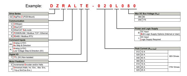
DigiFlex® Performance $^{\text{TM}}$  series of products are available in many configurations. Note that not all possible part number combinations are offered as standard drives. All models listed in the selection tables of the website are readily available, standard product offerings.
