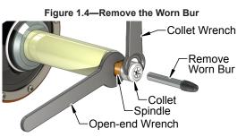
7. Insert the new bur leaving it out of the collet further than its initial position. Tighten the collet nut finger tight, so it snugs the bur in the collet. The bur should move with a little force, but stay in position when released.
