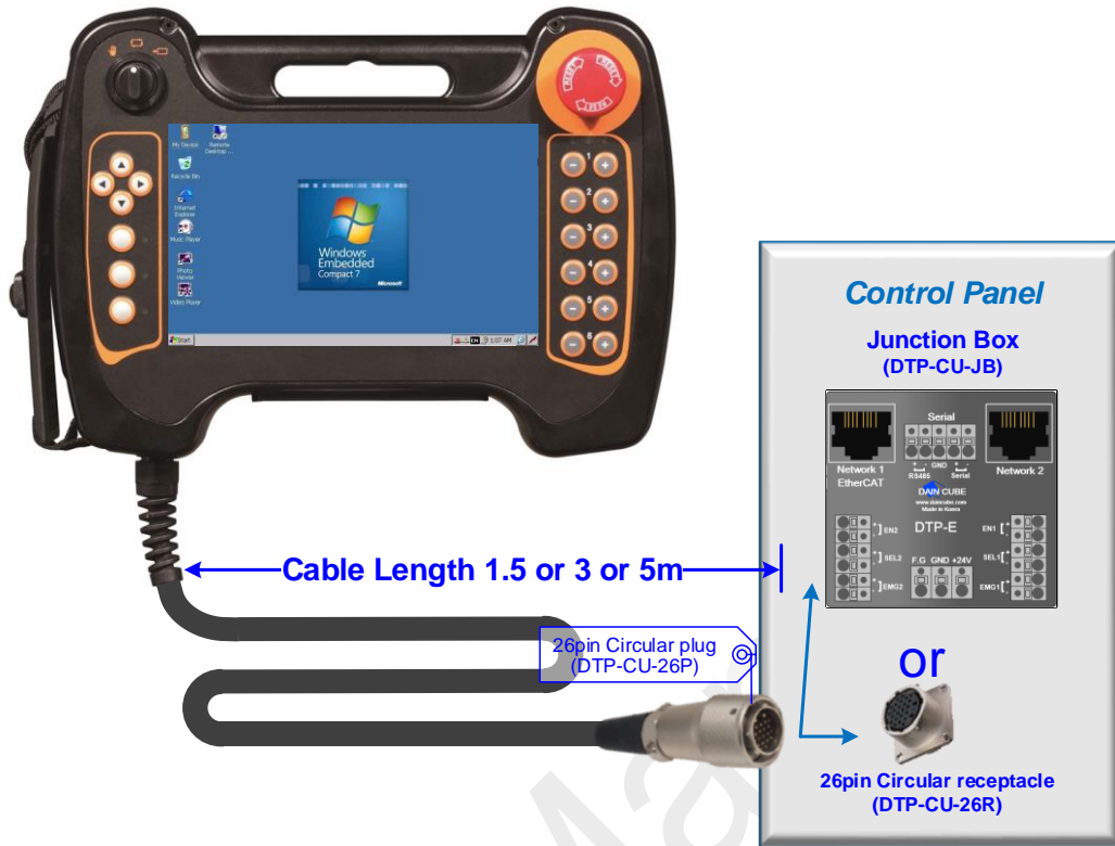
[Figure 8-3] Connections to junction box
