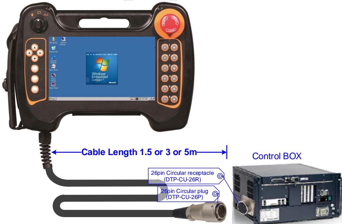
[Figure 8-4] Connections to Control Box
