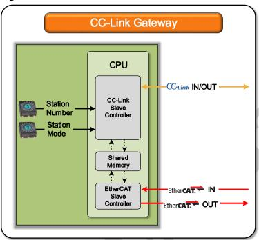
■ EtherCAT Master - CC-Link Master connection configuration diagram
