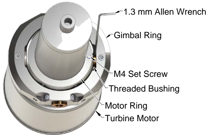
Figure 6.5—Motor Ring Bushing Adjustment
