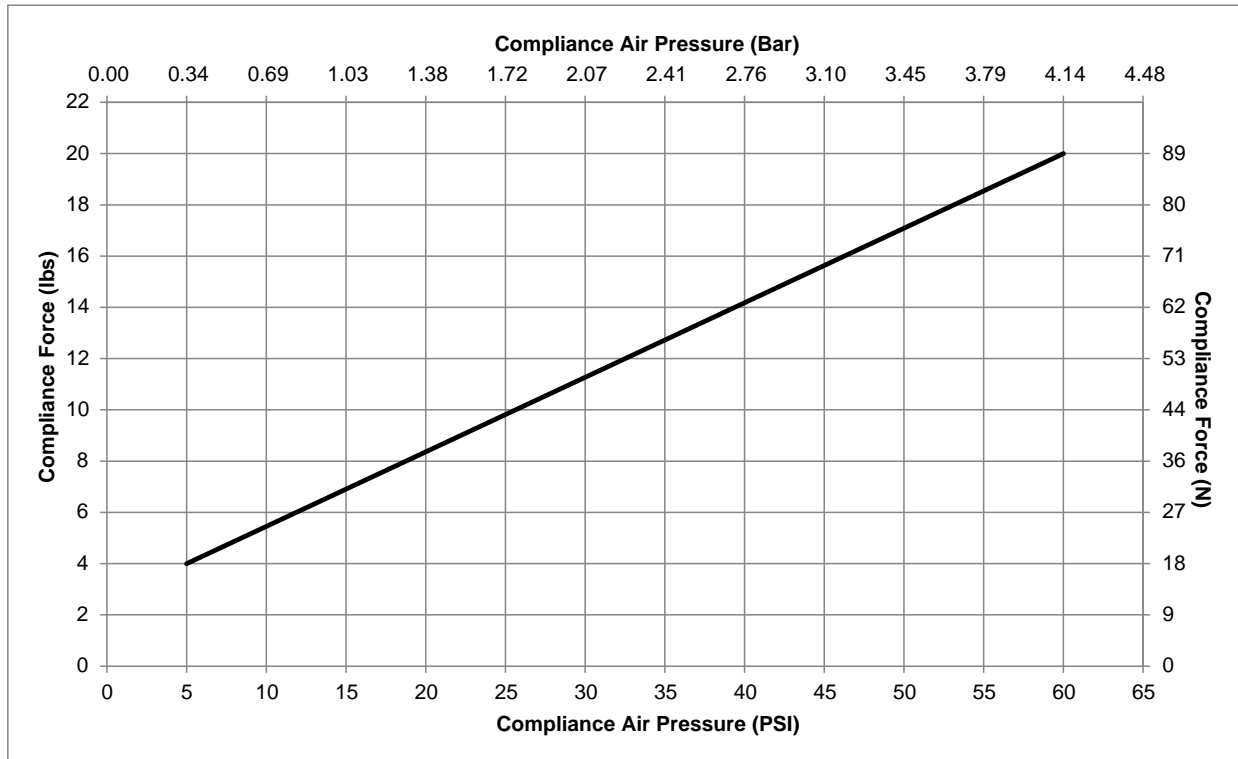
Figure 2.2—RC-1000 Series Radial Compliance Force (Measured at the Spindle Tip)
