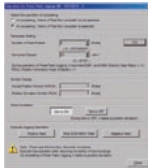
Pulse Feed Jogging: Simplifies motor operation and the entering of distance and travel speed data from a PC
